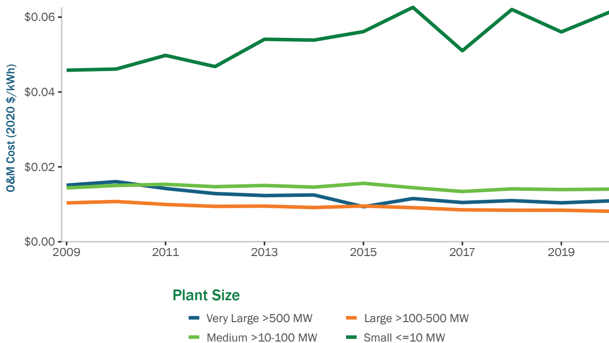
Figure 37. Trend in O&M cost per kilowatt-hour for utility-owned hydropower and PSH plants by size category (at average 2009–2020 capacity factor for each category)
